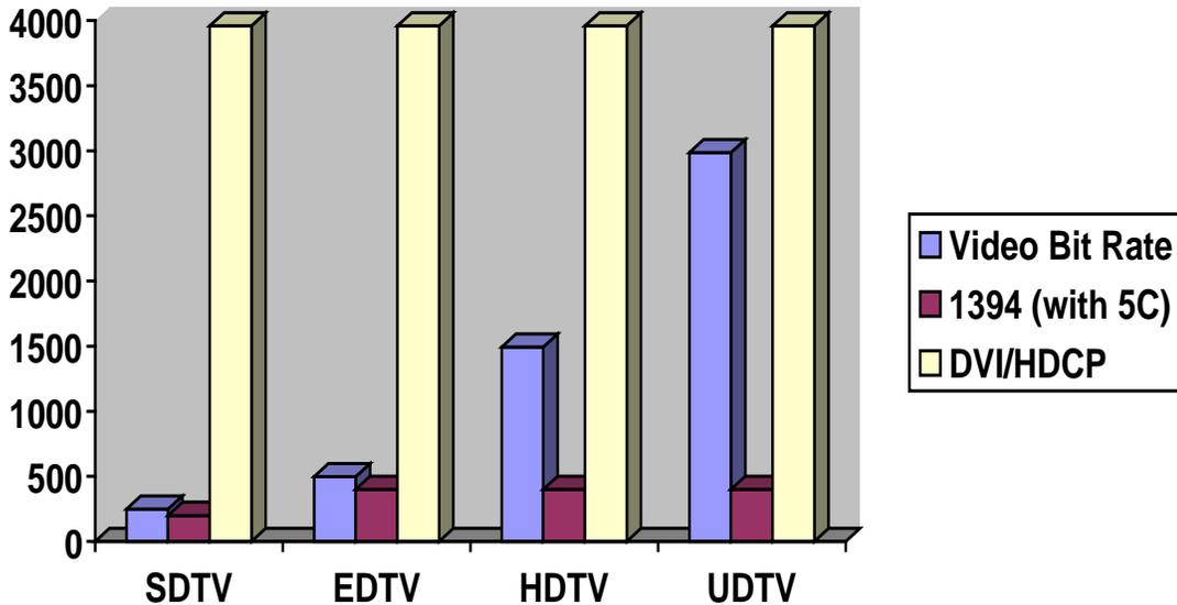
The above graph clearly indicates the inadequacy of the 1394 interface for certain applications and the capability of the DVI interface to handle current applications and beyond.
